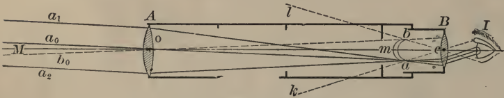
FIG. 8. — Path of the Rays in the Astronomical Telescope.
